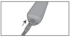
Insert the AC cord into the power supply.
