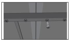
2 Secure the Base Pieces to each other using the eight hex bolts (four hex bolts for each Connecting Rod) making sure to hand tighten each and then tighten 1/4 turn more, as over-tightening could cause damage to the frame or Connecting Rod.
